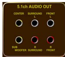
Diagram 1. 5.1ch Audio Connection DVD Player and A/V Amplifier
